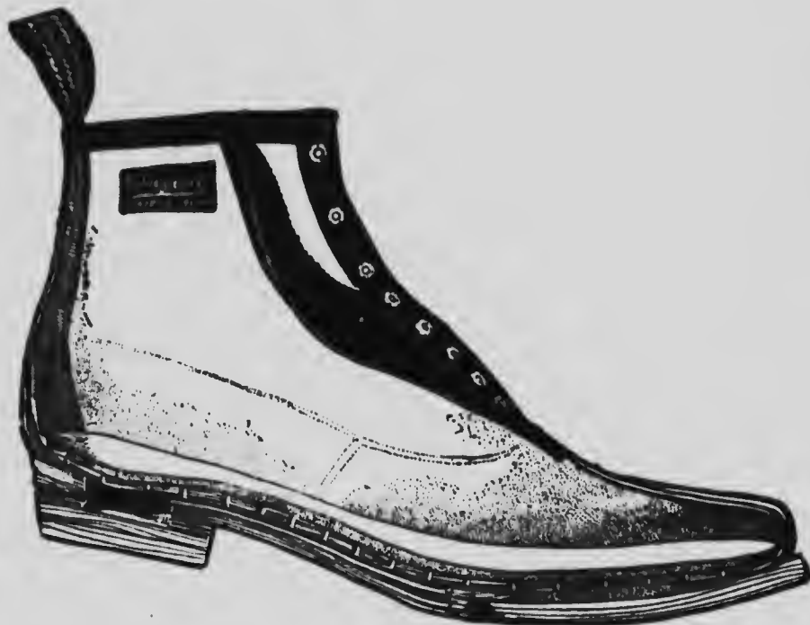
Showing Patent Ventilating System running along the Sole, and through the Heel, to the outer air.
